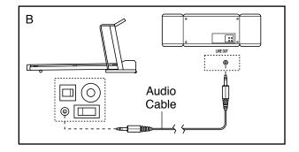
C. Plug one end of the audio cable into the jack on the front of the treadmill near the power cord. Plug the other end of the cable into a 3.5mm Y-adapter (available at electronics stores). Plug the Y-adapter into the PHONES jack on your stereo. Plug your headphones into the other side of the Y-adapter.
